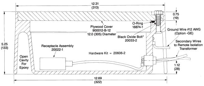
\* Typical for 6 bolts equally spaced on 11.25 (286) diameter bolt circle
